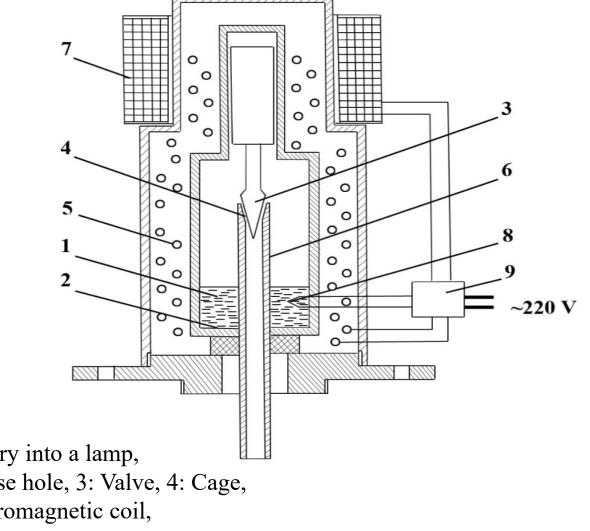
Figure 1. Device for dosing mercury into a lamp,
