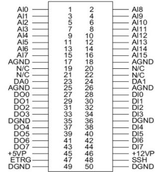
Figure 5. Connector 50 pin of DAQ card
