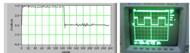
Figure 29. Square wave applied to the load and sampled wave form
