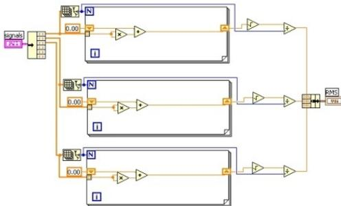
Figure 15. RMS value calculated under the program and the voltage drop
