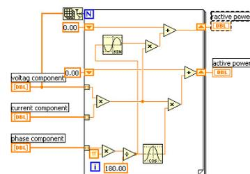
Figure 20. Block diagram under the program can calculate the active and reactive
