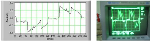
Figure 32. All-wave rectifier current wave form control with all the fire angle of 60 degrees
