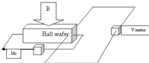
Figure 3. Hall generator diagram
