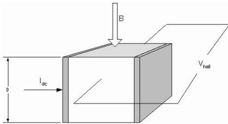
Figure 2. Hall Effect in semiconductor wafer
