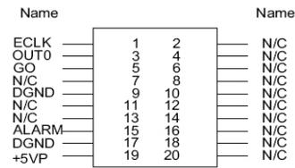
Figure 6. Connector 20 pins of DAQ card
