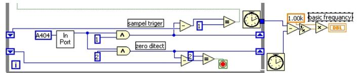
Figure 18. How to determine the basic frequency
