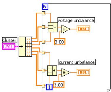
Figure 16. Block diagram of calculation unbalanced of voltage and current signal
