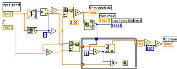
Figure 10. Block diagram to calculate the FFT
