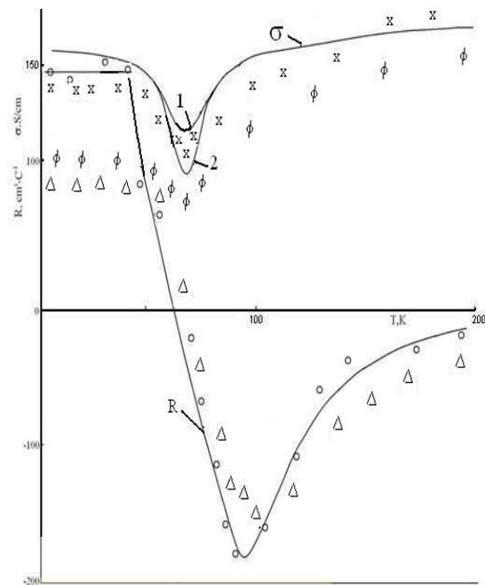
Figure 1. Temperature relationships of electric conduction  $\sigma$  and Hall coefficient  $R$  in p- $\text{Ag}_2\text{Te}$ ,
