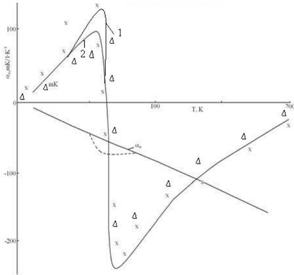
Figure 2. Temperature relationship of thermo electromotive force  $\alpha_0(T)$  in p-Ag<sub>2</sub>Te. Experimental points: symbols are the same as in Figure 1 and solid lines are design ones for concentration of  $p' = 4.2 \times 10^{16} \text{ cm}^{-3}$
