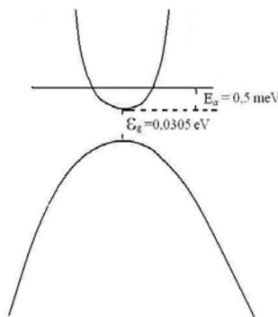
Figure 4. Zone structure of p-Ag<sub>2</sub>Te at  $T=65\text{K}$
