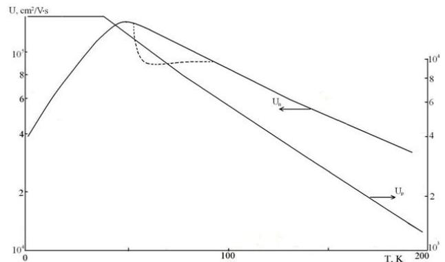
Figure 3. Temperature relationship of electron  $U_n(T)$  and hole  $U_p(T)$  mobility in p-Ag<sub>2</sub>Te, Dotted lines are due to electron scattering on acceptor centres
