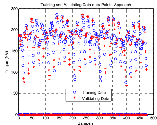
Figure 10. Separating the data in Points method (There are 292 Points for training and 183 Points for the evaluation of the ANN model)
