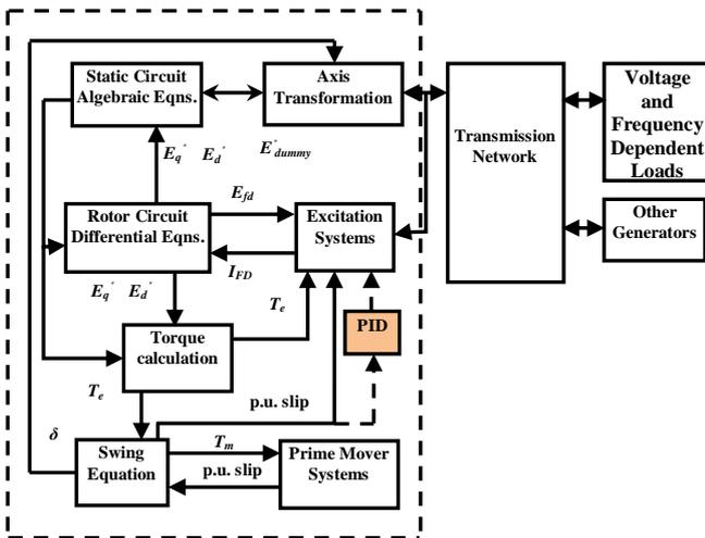
Figure 1. Structure of PSS in power systems [5]
