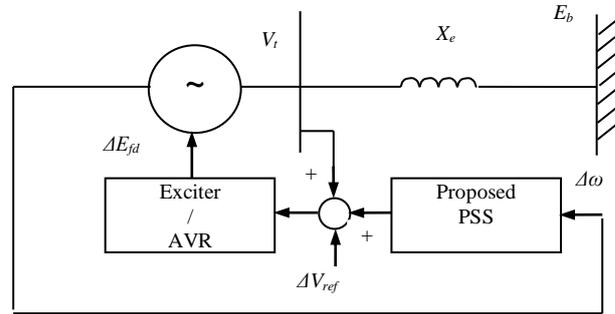
Figure 2. Schematic diagram of single machine infinite bus system [1]
