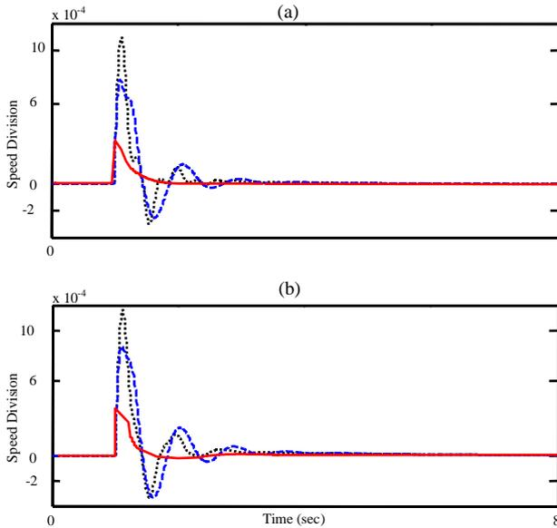
Figure 10. System response by applying a 6-cycle three-phase fault at  $t=1$ : Solid (MSF- PSOTVAC), Dashed (GA-PSS) Doted (CPSS)
