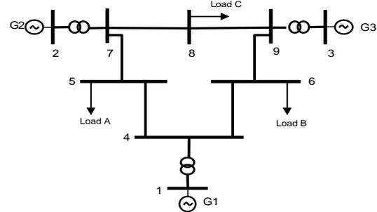
Figure 3. Three-machine nine-bus power system [5]
