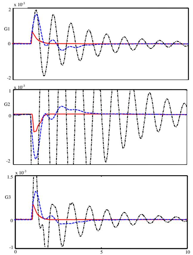
Figure 12. System response under scenario 1 with heavy loading condition: Solid (MSF- PSOTVAC) Dashed (PSOPSS) Doted (CPSS)
