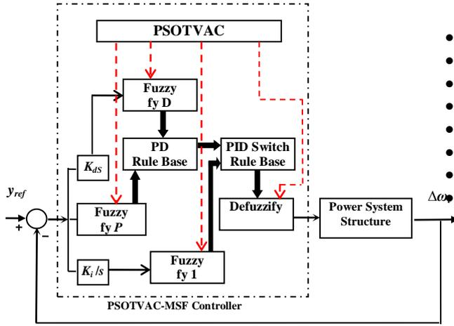
Figure 5. Structure of the proposed controller [14]
