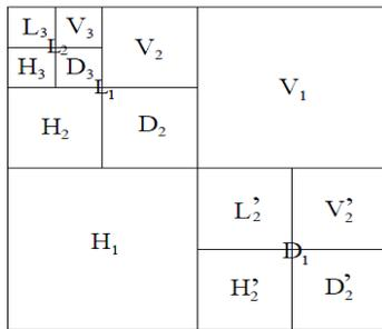
Figure 4. The sub bands resulted from wavelet decomposition [5]
