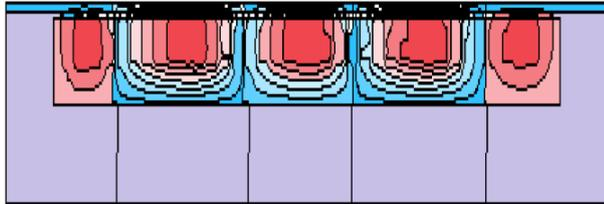
Figure 4. Finite element calculation equipotential lines (B lines)
