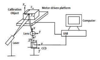
Figure 1. The block diagram of the 3D scanning with handheld Laser and Webcam - DAVID Laser scanner v3 [6]
