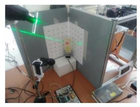
Figure 10. Implemented 3D scanner
