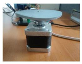
Figure 7. Platform mounted NEMA17 stepper motors
