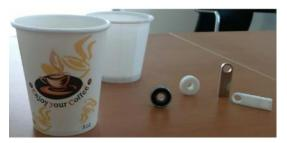
Figure 16. Original objects and their reproductions using proposed 3Dscanner/printer
