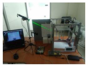
Figure 11. Implemented 3D scanner with 3D printer unit.
