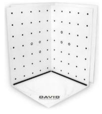
Figure 2. The calibration patterns [12]
