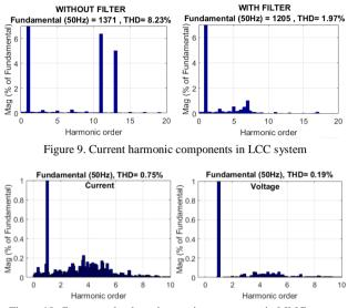
Figure 10. Current and voltage harmonic components in MMC system
