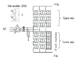
Figure 2. MMC principle scheme [9]
