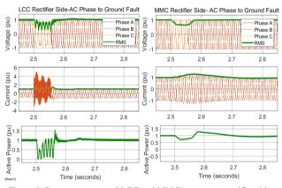
Figure 5. System response of LCC and MMC converters rectifier sides during A-G fault
