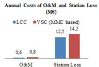
Figure 12. Station loss and O&M costs of both converters [12]
