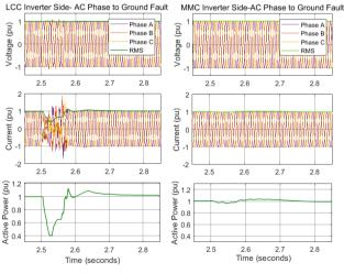
Figure 7. System response of LCC and MMC converters inverter sides during A-G fault
