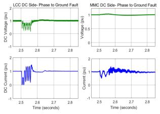
Figure 6. DC voltages and currents of LCC and MMC during A-G fault
