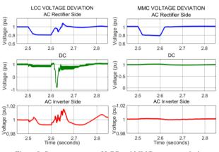
Figure 8. System response of LCC and MMC converters during voltage deviations
