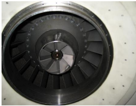
Figure 1. Typical Hybrid burner assembly HR3 - type, for dual fuel operation
