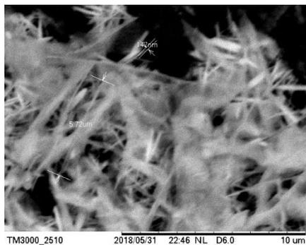
Figure 2. The nanorods observed in the PbSe thin film
