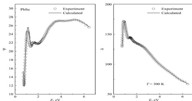
Figure 3. The main angles of ellipsometry  $\Psi$  and  $\Delta$  of the PbSe thin film
