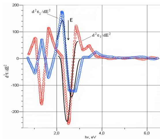
Figure 5. Spectral dependencies of the second derivatives of the  $\epsilon_1(\omega)$  is real and  $\epsilon_2(\omega)$  is imaginary parts of the complex dielectric function (respectively shown in red and blue circles) and the best fittings curves constructed by "Graphical analysis" program for 2÷3 eV energy region (solid lines) of the nanostructured PbSe thin film
