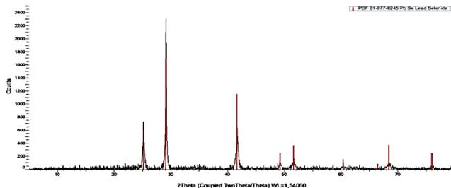
Figure 1. X-ray diffraction spectrum of PbSe thin film
