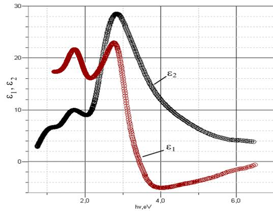
Figure 4. Spectral dependencies of the  $\epsilon_1(\omega)$  is real and  $\epsilon_2(\omega)$  is imaginary parts of the complex dielectric function of the nanostructured PbSe thin film
