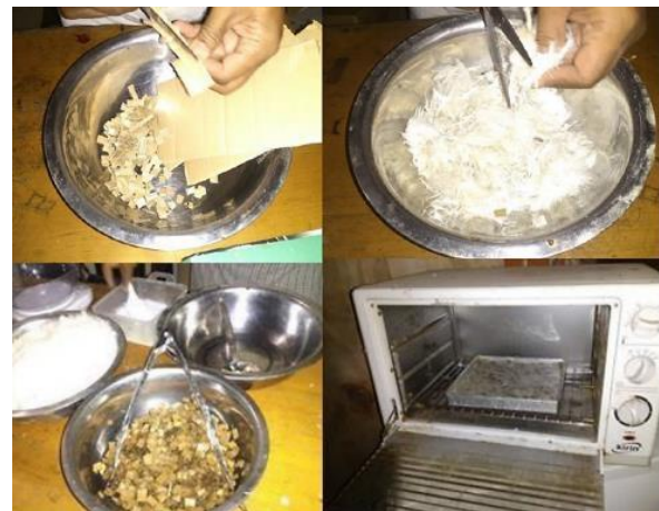
Figure 2. Waste chicken feathers and cardboard used as acoustic panel material [7]
