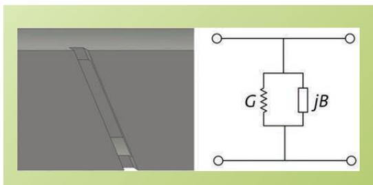
Figure 2. Inclined slot design [2]
