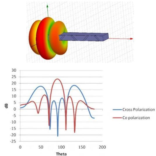
Figure 5. Modelled structure with 2 slots [HFSS Simulation Results]
