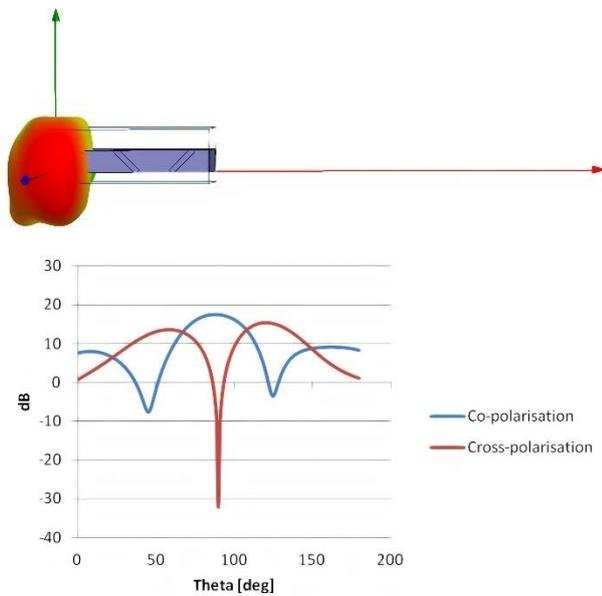
Figure 4. Modelled structure with 2 slots [HFSS Simulation Results]
