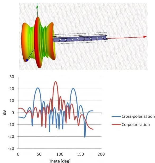
Figure 5. Modelled structure with 2 slots [HFSS Simulation Results]
