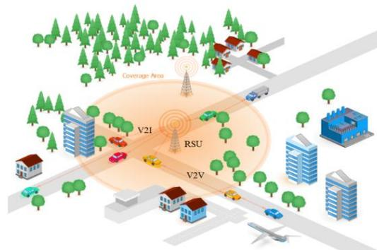
Figure 1. VANET network architecture
