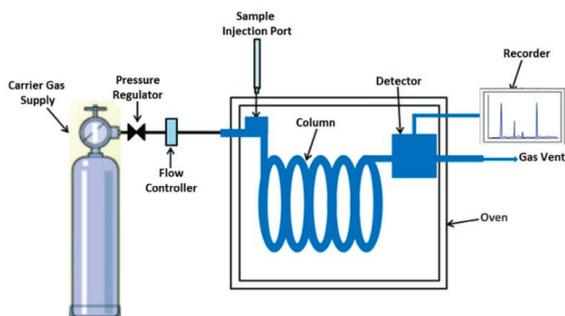
Figure 1. Basic gas chromatograph [10]
