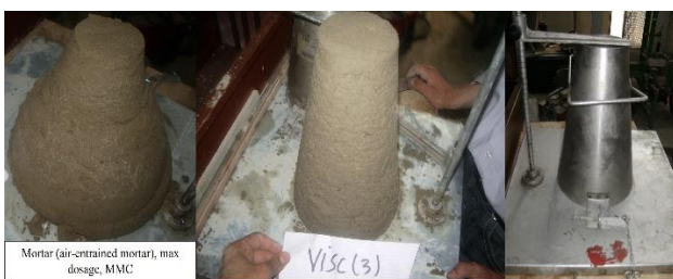
Figure 1. Abram’s cone slump tests
