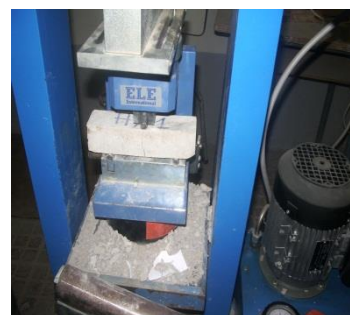
Figure 5. Tensile strength tests (by bending)
