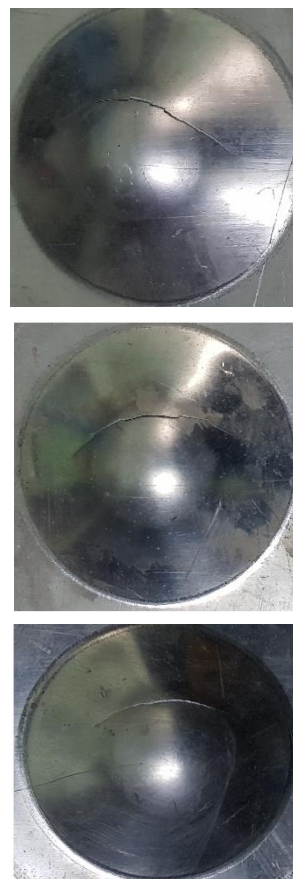
Figure 1. the position and size of the necking for three different specimens using different forming speeds
