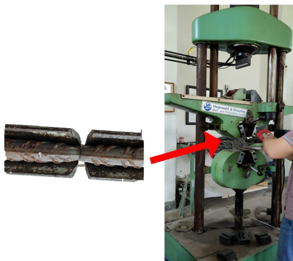
Figure 1. Universal testing machine DLY-30 and rebar sample photo selected randomly during measurements
