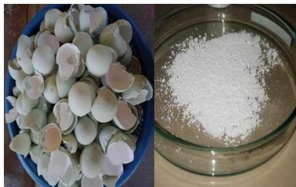
Figure 2. Egg shells, the basic material for producing catalysts: a. egg shell; b. CaO/Na/ \gamma -Al 2 O 3
