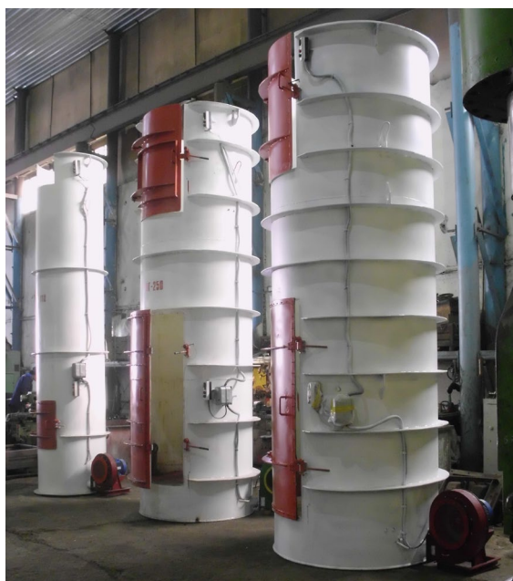
Figure 10. Pneumatic lifts with a lifting capacity of 110, 250, 500 Kg [2]
