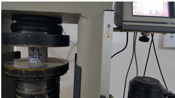
Figure 9. Concrete compressive strength, K1 at B9
