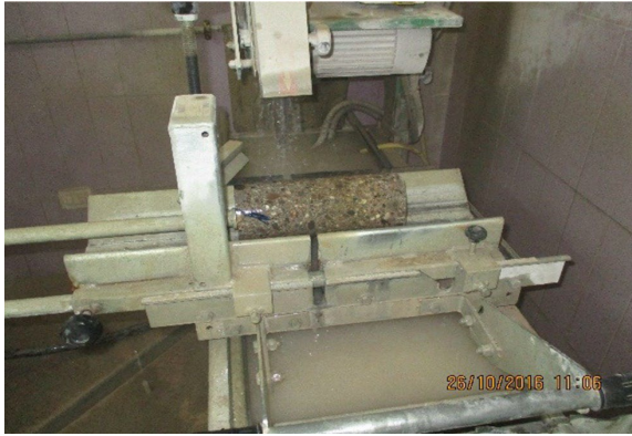
Figure 8. Cutting device for concrete sample preparation
