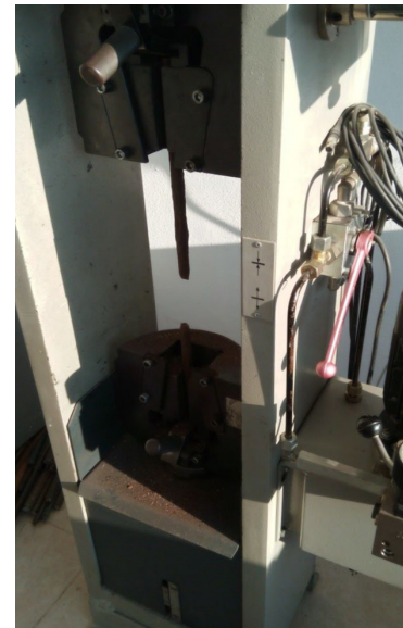
Figure 10. Tensile test of the steel bar sample
