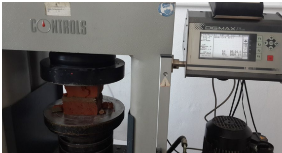
Figure 13. Masonry compressive strength test
