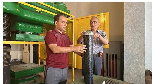
Figure 3. Visual analysis of the post-disintegration condition of a triple carbon fiber-clad element
