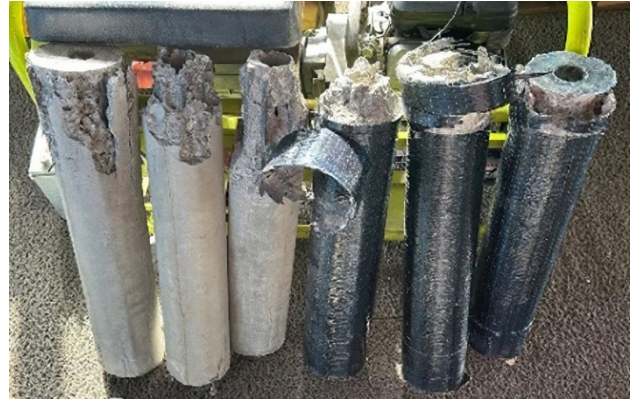
Figure 4. Condition of the tested elements after disintegration
